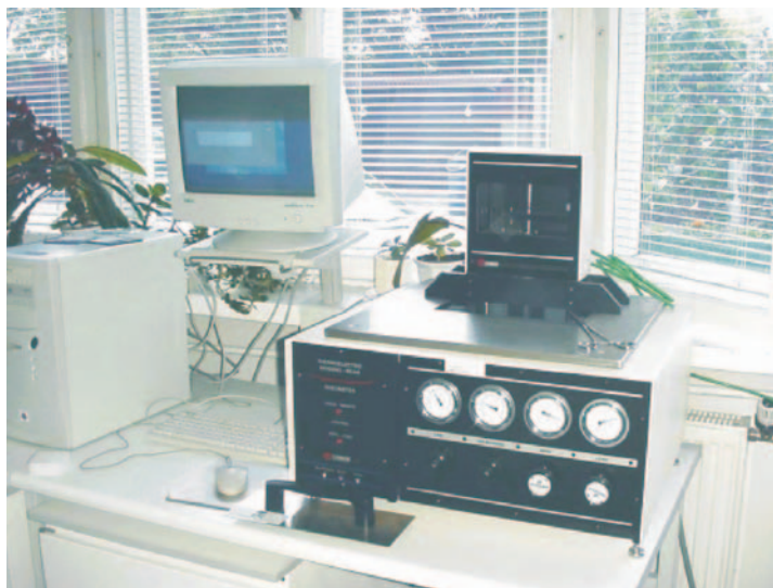
Rys.3. Reometr BBR w laboratorium IBDiM Fig.3. BBR rheometr at IBDiM laboratory
