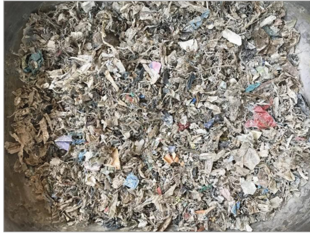
Fig. 3. IP10-Ca mixture composed of lime and shredded waste from group 19 12 12
