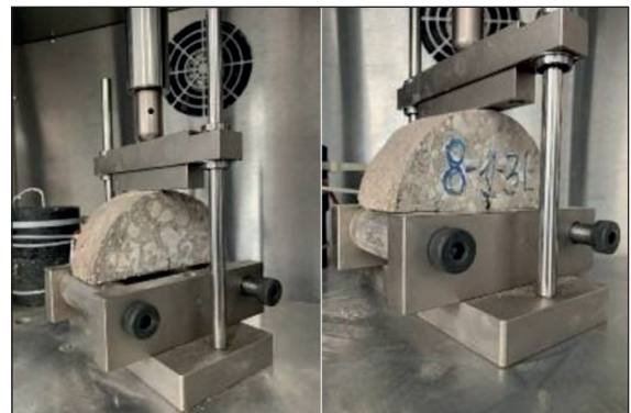
Fig. 24. SCB (Semi-Circular Beam) test; photo: J. Krasowski
