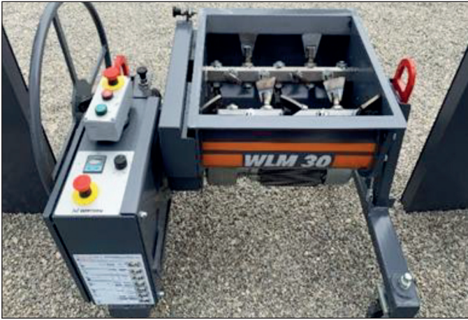
Fig. 10. Wirtgen WLM 30 laboratory mixer; photo: J. Krasowski
