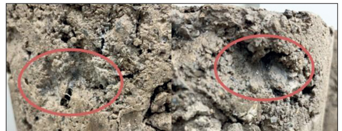
Fig. 6. Visible polymer network structure on CBGM mix specimens; photo: M. Krasowski
