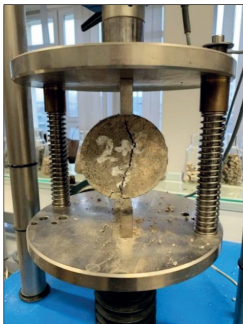
Fig. 15. Indirect tensile strength test used for calculate ITS_{DRY} ; photo M. Krasowski
