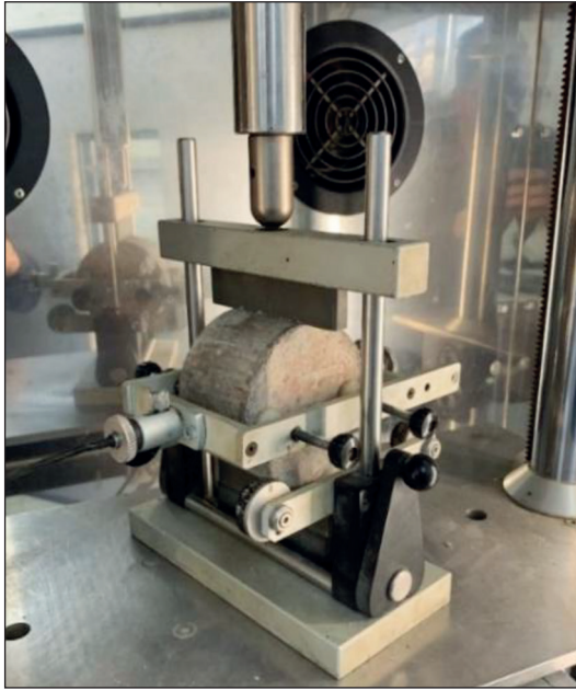
Fig. 19. Test RIG for IT-CY stiffness modulus tests; photo M. Krasowski
