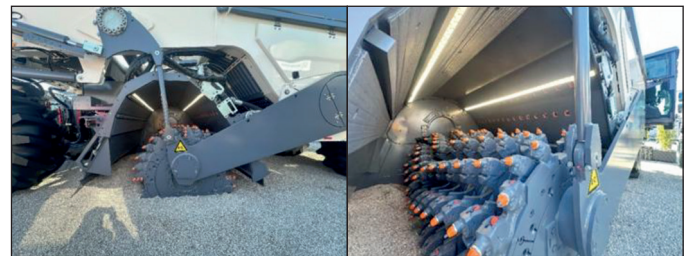
Fig. 2. Mixing drum of the Wirtgen WR 200i recycler; photo: M. Krasowski
