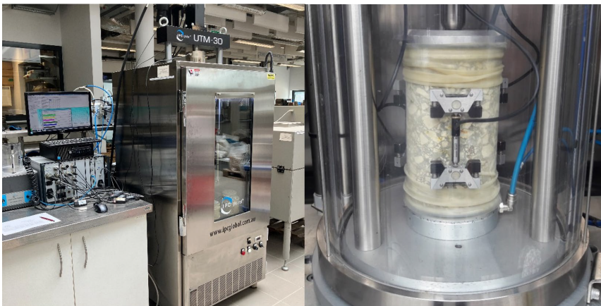
Fig. 2. On the left, the IPC Global UTM-30 machine used in the tests, on the right, a sample during the testing of the dynamic complex stiffness modulus
