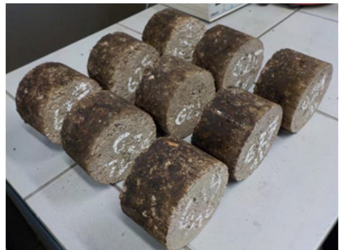
Fig. 4. Samples for ITS tests
