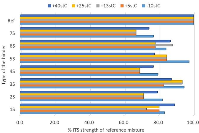
Fig. 12. Indirect tensile strength – coarse-grained MCE mixture
