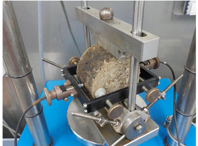
Fig. 3. Loading scheme in IT-CY tests
