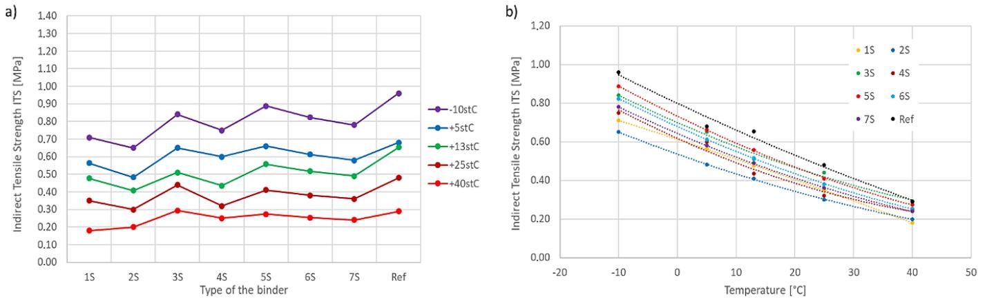
Fig. 11. Indirect tensile strength – fine-grained MCE mixture: a) binder dependency; b) temperature dependency
