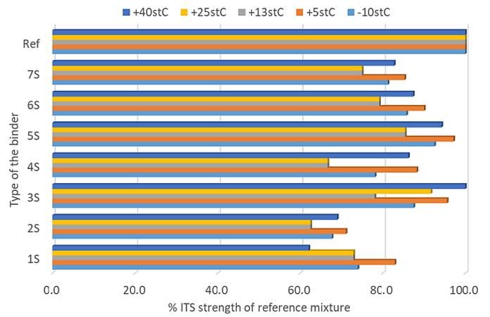
Fig. 13. Indirect tensile strength – fine-grained MCE mixture
