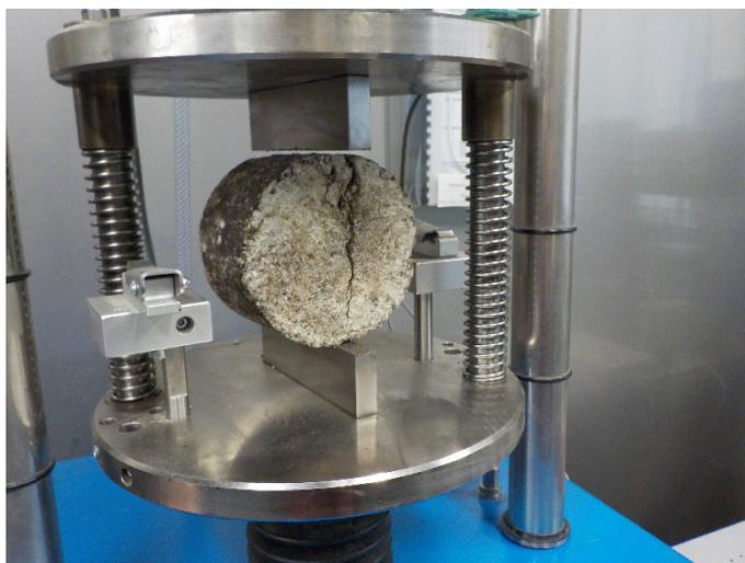
Fig. 5. Scheme of ITS tests
