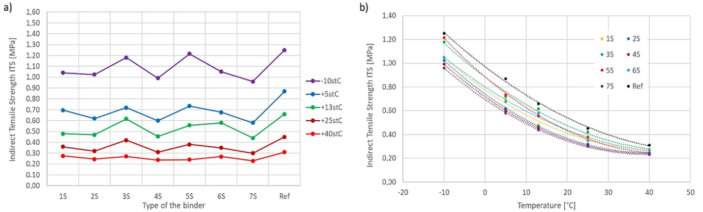
Fig. 10. Indirect tensile strength – coarse-grained MCE mixture: a) binder dependency; b) temperature dependency
