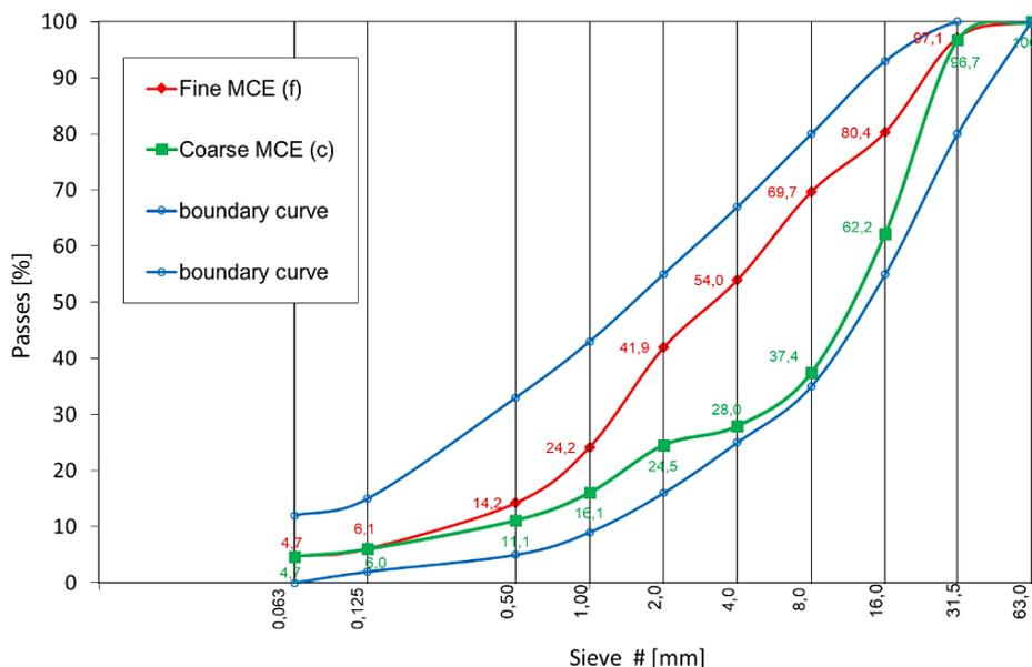
Fig. 1. Graining curves of mineral mixtures (MM)
