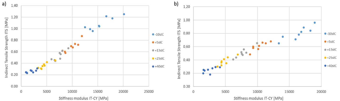
Fig. 14. Dependence of the indirect tensile strength (ITS) on the stiffness modulus (IT-CY) MCE mixture: a) coarse-grained; b) fine-grained
