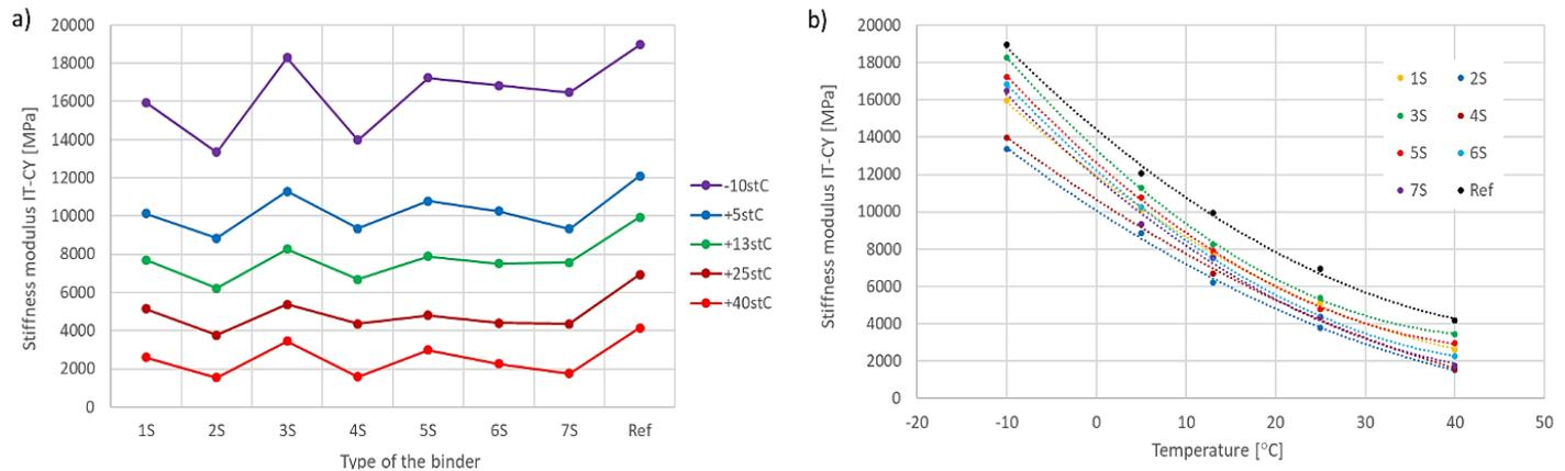
Fig. 7. IT-CY Stiffness modulus – fine-grained MCE mixture: a) binder dependency; b) temperature dependency
