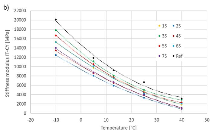
Fig. 6. IT-CY Stiffness modulus – coarse-grained MCE mixture: a) binder dependency; b) temperature dependency
