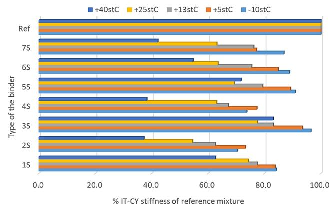
Fig. 9. Reduction of the IT-CY stiffness modulus – fine-grained MCE mixture
