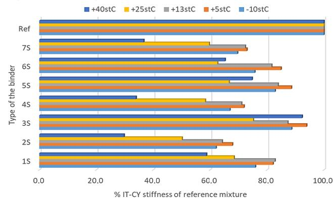
Fig. 8. Reduction of the IT-CY stiffness modulus – coarse-grained MCE mixture
