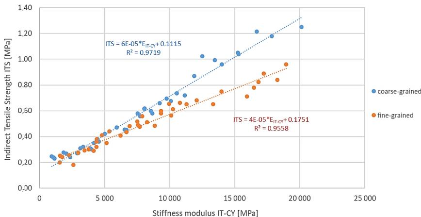
Fig. 15. Dependence of the indirect tensile strength (ITS) on the stiffness modulus (IT-CY) for coarse-grained and fine-grained MCE mixtures in the tested temperature range
