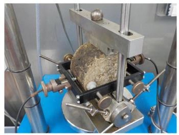
Fig. 3. Loading scheme in IT-CY tests
