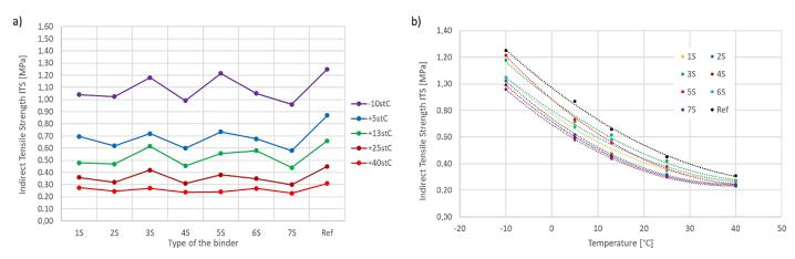
Fig. 10. Indirect tensile strength - coarse-grained MCE mixture: a) binder dependency; b) temperature dependency
