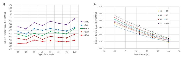
Fig. 11. Indirect tensile strength - fine-grained MCE mixture: a) binder dependency; b) temperature dependency
