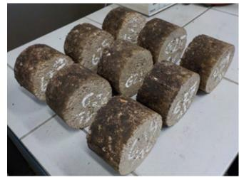
Fig. 4. Samples for ITS tests
