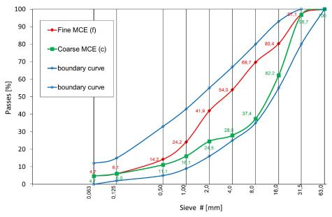
Fig. 1. Graining curves of mineral mixtures (MM)
