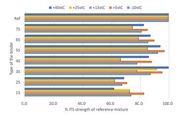
Fig. 13. Indirect tensile strength - fine-grained MCE mixture
