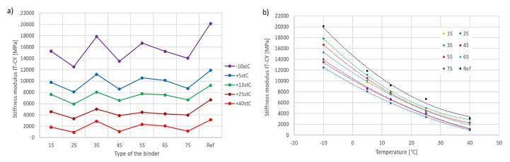
Fig. 6. IT-CY Stiffness modulus - coarse-grained MCE mixture: a) binder dependency; b) temperature dependency
