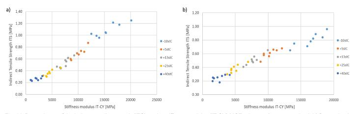
Fig. 14. Dependence of the indirect tensile strength (ITS) on the stiffness modulus (IT-CY) MCE mixture: a) coarse-grained; b) fine-grained
