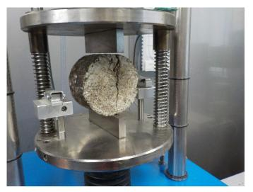
Fig. 5. Scheme of ITS tests
