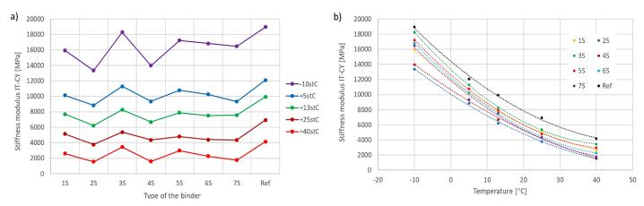
Fig. 7. IT-CY Stiffness modulus - fine-grained MCE mixture: a) binder dependency; b) temperature dependency
