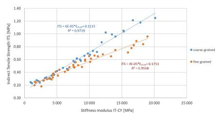
Fig. 15. Dependence of the indirect tensile strength (ITS) on the stiffness modulus (IT-CY) for coarse-grained and fine-grained MCE mixtures in the tested temperature range
