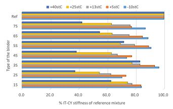
Fig. 9. Reduction of the IT-CY stiffness modulus – fine-grained MCE mixture
