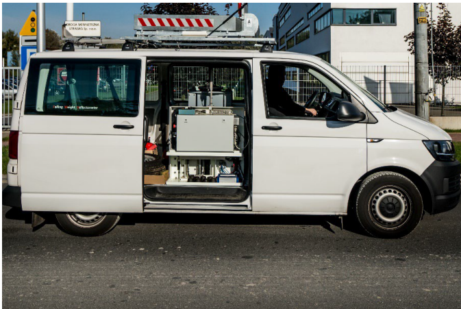
Fig. 5. Testing the pavement load-bearing capacity using a Falling Weight Deflectometer (FWD)
