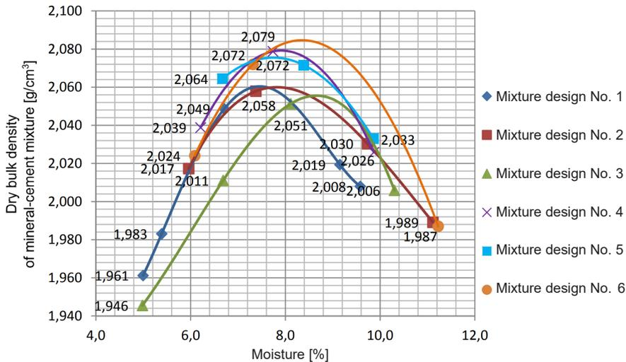
Fig. 2. Determination of the optimal moisture of the designed mineral-cement mixtures [5]
