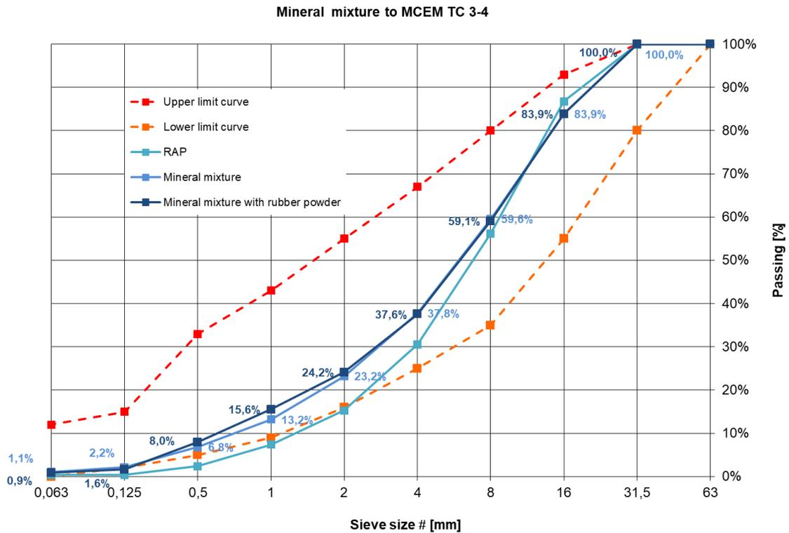
Fig. 5. MCEMRP1 coarse-grained with 0/1 mm rubber powder at the lower grain size fraction < 4 mm for medium traffic category TC3÷4
