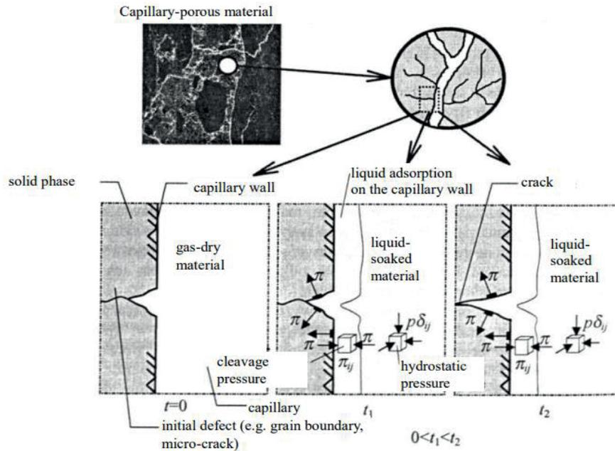
Fig. 3. Graphical diagram of the Rebinder effect - action of cleavage forces [21]
