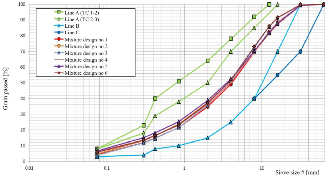
Fig. 1. Graining of mineral-cement mixtures [5]
