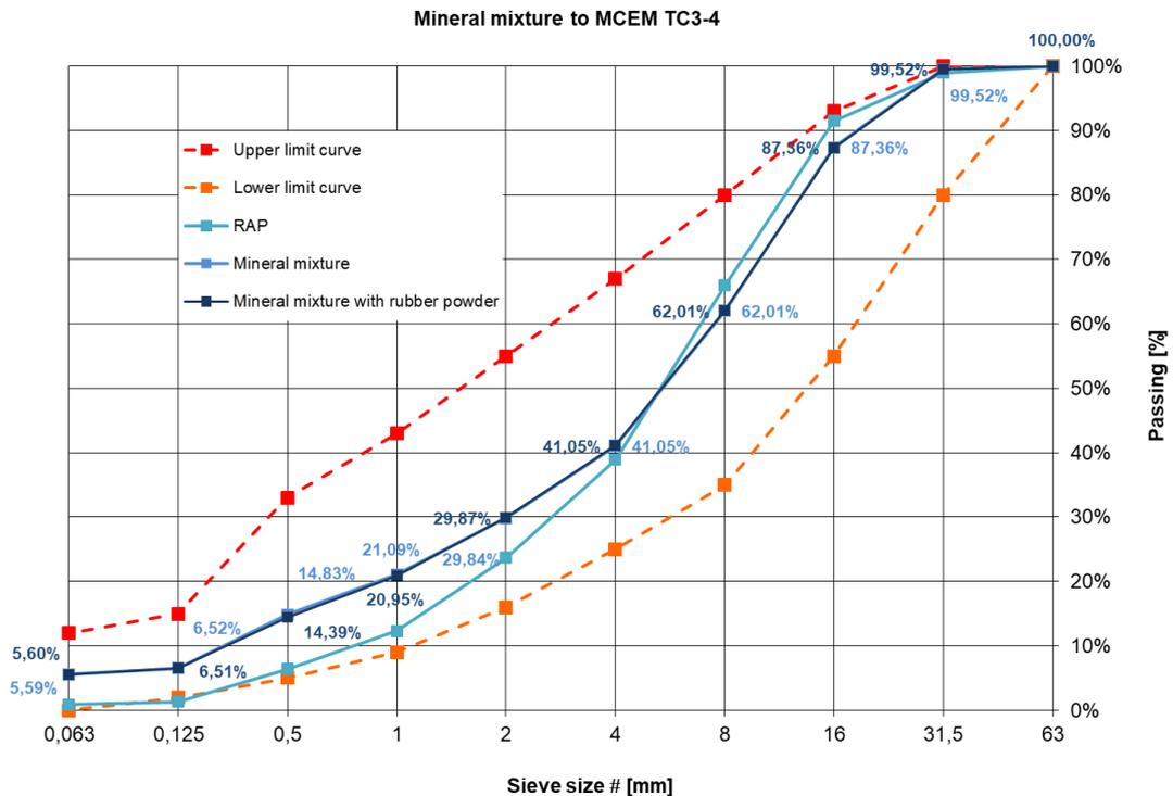
Fig. 6. MCEMRP2 medium-grained with 0/1 mm rubber powder in the middle position between the limit curves for medium traffic category TC3÷4
