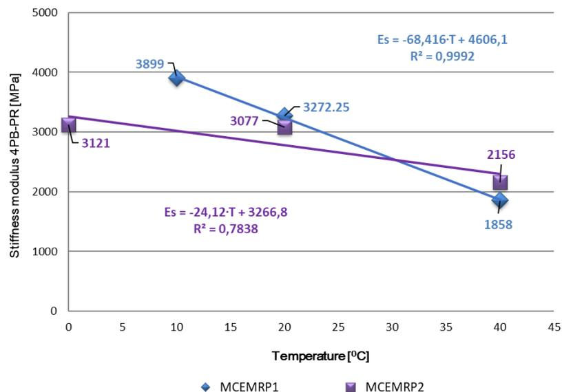
Fig. 7. Correlation between temperature and the stiffness modulus of the beams at the lower grain limit of MCEMRP1 and the middle position between the grain limit curves of MCEMRP2
