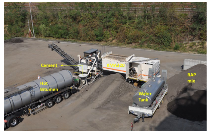
Fig. 6. Production of the cold recycled mix with mobile plant (KMA 220)
