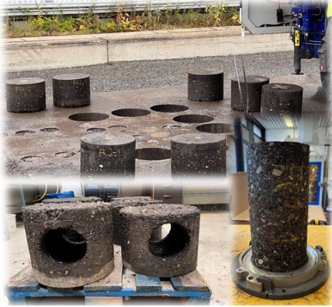
Fig. 28. 50 cm diameter cores and the side coring to prepare 3 axial test specimens
