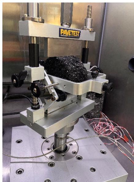
Fig. 4. Stiffness modulus determination with IT-CY test on AC 16 W 50/70 specimens
