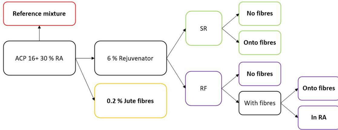
Fig. 2. Test plan scheme
