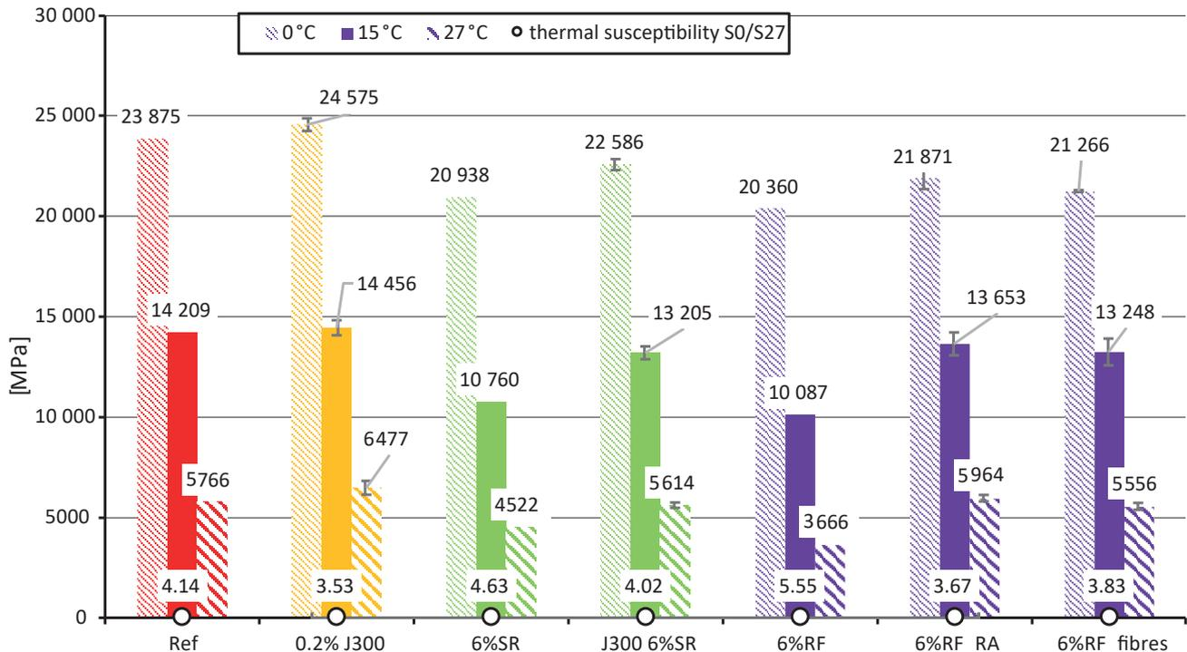
Fig. 5. Stiffness modulus results
