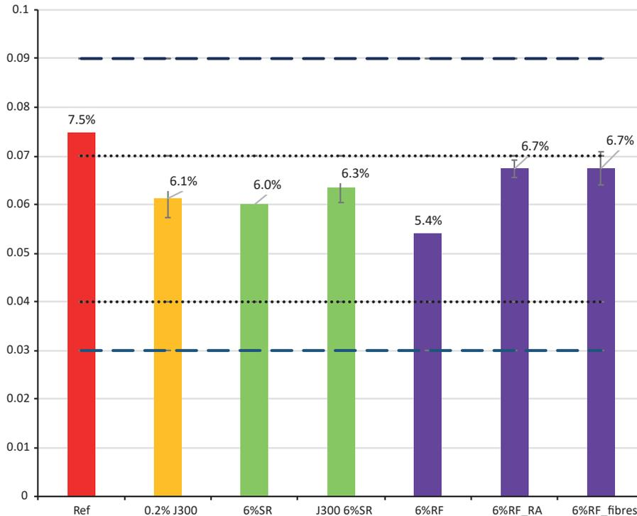
Fig. 3. Air voids content (the dotted lines show the interval for type testing limits, the dashed lines show the interval for control testing requirements in Czech Republic for AC<sub>base</sub> mixtures)
