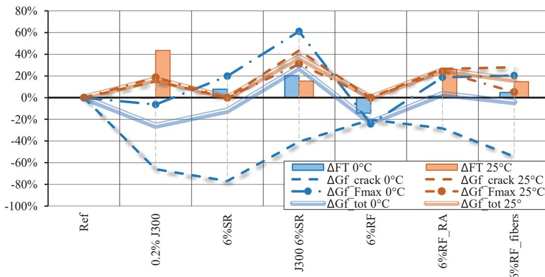
Fig. 7. Fracture parameters relative to the reference mixture (FT: Fracture Toughness, Gf\_Fmax: Energy to the maximum force, Gf\_tot: Total fracture energy)
