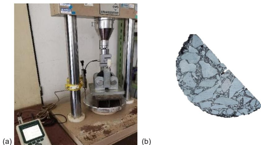
Fig. 6. (a) Semi-circular specimen, (b) SCB test setup
