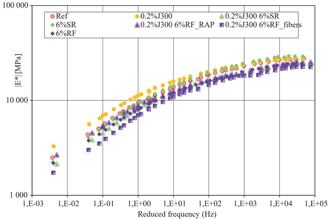
Fig. 8. Master curves for 4PB complex modulus of tested mix variants
