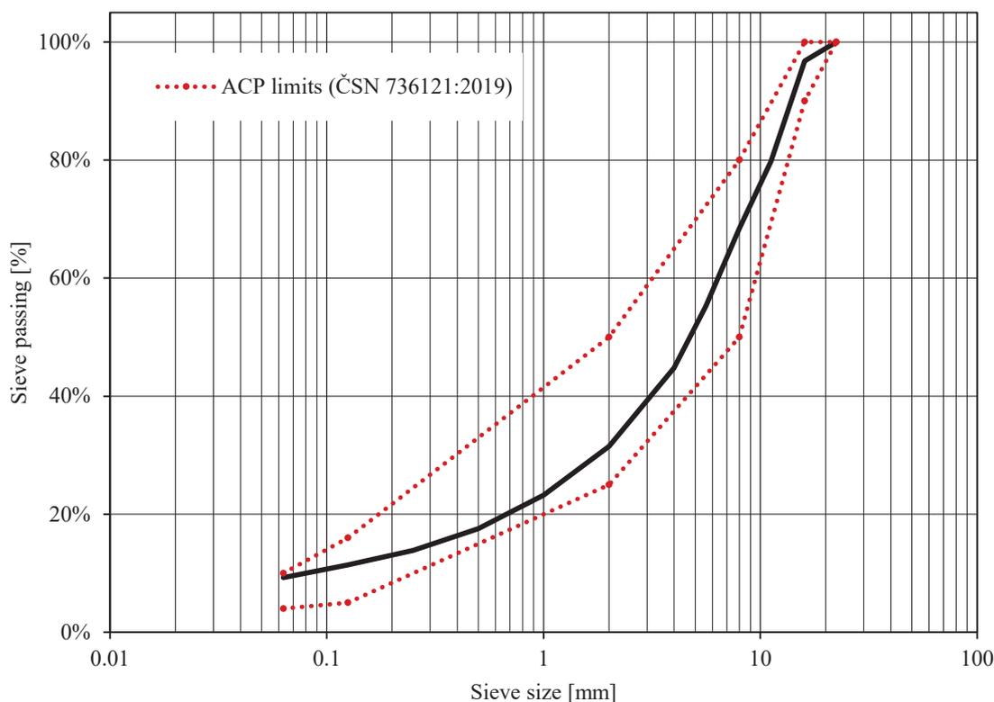
Fig. 1. Granulometric curve of the reference mixture
