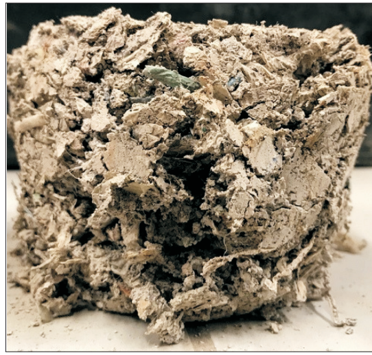
Fig. 18. Specimen after failure – mixture obtained by adding 300 kg of fragmented plastic waste to 1 m 3 of CBM
