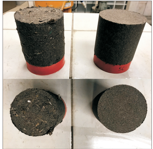
Fig. 6. Specimen with considerable content of fragmented plastic waste and a reference specimen
