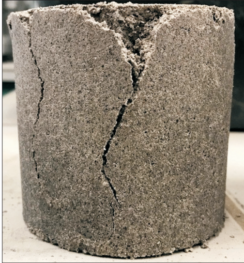
Fig. 15. Reference specimen (without fragmented plastic waste) after failure
