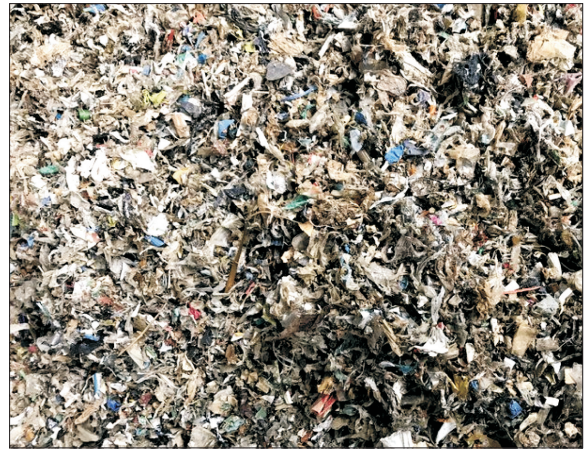
Fig. 1. Fragmented plastic waste with the bulk density of 1.195 \text{ g/cm}^3
