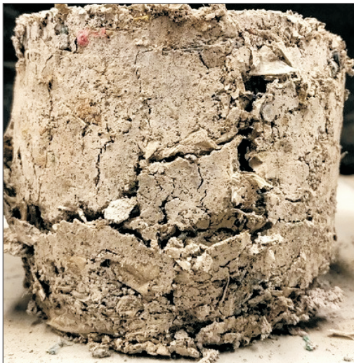
Fig. 17. Specimen after failure – mixture obtained by adding 200 kg of fragmented plastic waste to 1 m 3 of CBM
