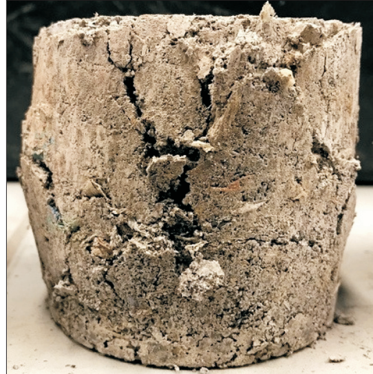
Fig. 16. Specimen after failure – mixture obtained by adding 100 kg of fragmented plastic waste to 1 m 3 of CBM
