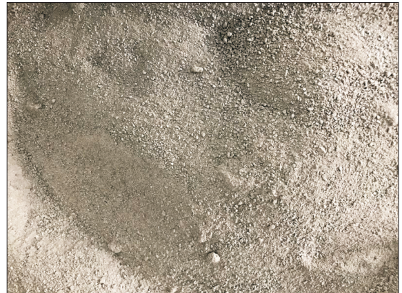
Fig. 2. The used 0/2 mm granodiorite aggregate Rys. 2. Kruszywo granodiorytowe 0/2 mm
