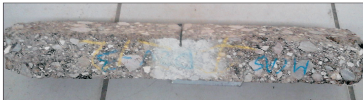
Fig. 1. Notched specimen for the 4PB-PR test
