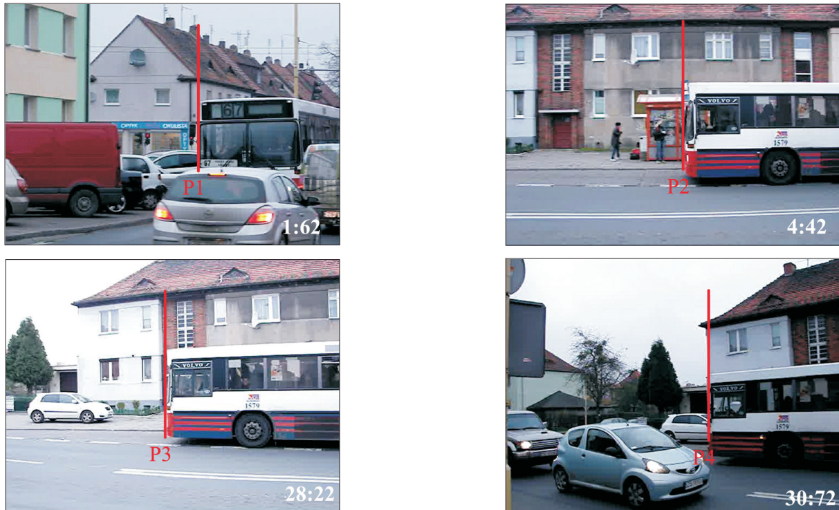
Fig. 2. Visualization of shortened way of measuring bus drive through times by means of video camera with detailed time recording function; between points P2 and P3 bus approach time (3.00 s) and stoppage time (20.80 s) were taken into account
