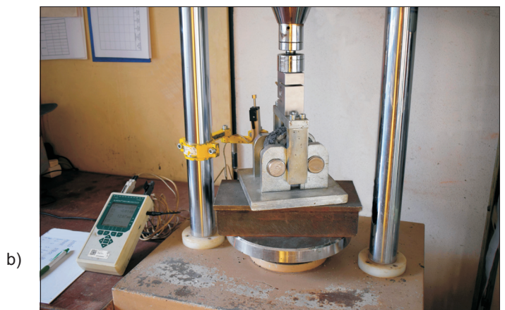
Fig. 1. Modified semi-circular bending test (SCB test): a) geometry of equipment, b) view of measuring devices
