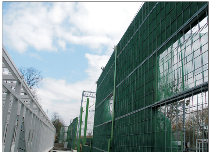
Fig. 4. The first investigated section: from the left (direction of incoming trains) a span with removed panels, the tested span no. 1-2 with visible damaged middle panel and accelerometers (installed on the top of the columns and the panel), and an adjacent span with two damaged panels
