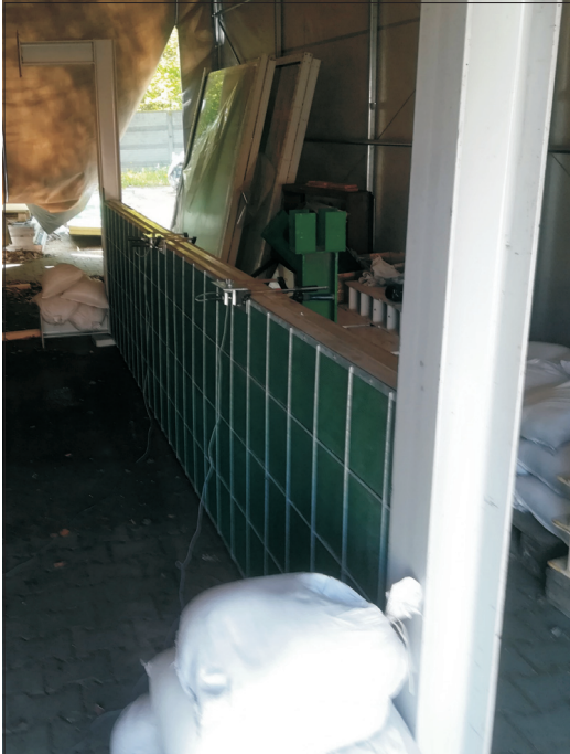
Fig. 19. Vertically installed panel during dynamic testing using modal impact hammer; accelerometers mounted on the top part of the panel
