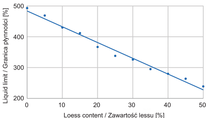
Fig. 1. Influence of loess content on the liquid limit of the bentonite-loess mixtures
