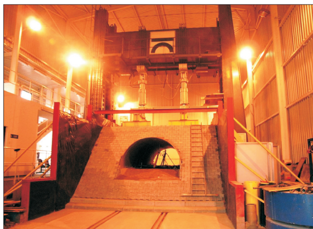
Fig 3. Full-scale test of soil-shell structure load-bearing capacity (photo by R. Gut, 2017)
