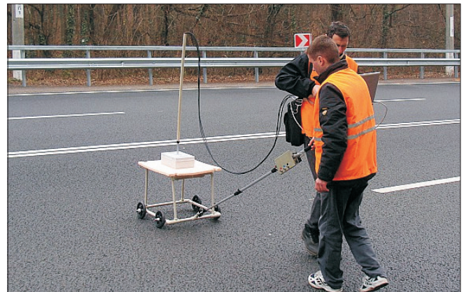
Fig. 3. GPR diagnostics of the pavement - transverse profile scanning
