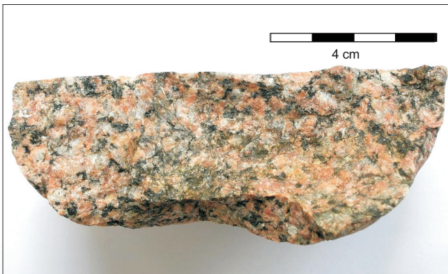
Fig. 5. Phaneritic, medium-grained granite (stereoscopic image on the right)
