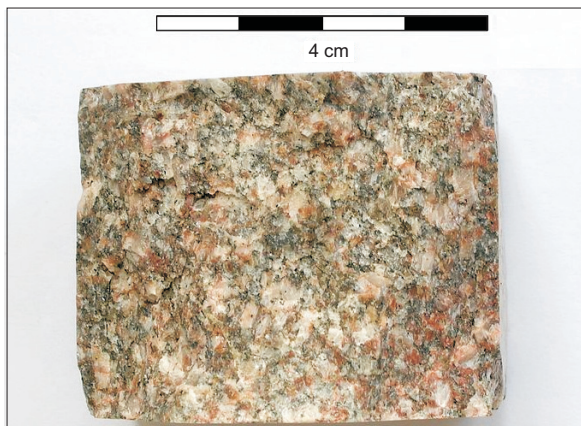
Fig. 6. Phaneritic, medium-grained granite (stereoscopic image on the right)
