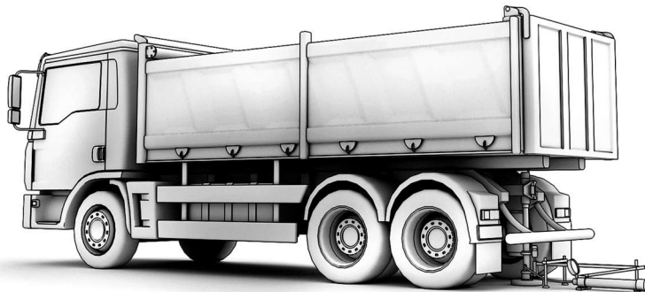
Fig. 3. Static plate load test carried out with the use of a heavy truck
