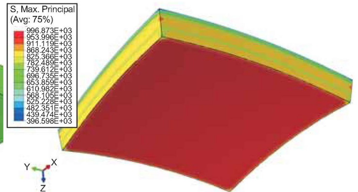
Fig. 13. Contours of maximum principal stresses in concrete plate - III variant (temperature loading, contact)
