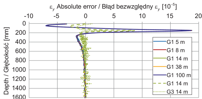
Fig. 11. The absolute error of vertical deformations \varepsilon_y in hemispherical models
