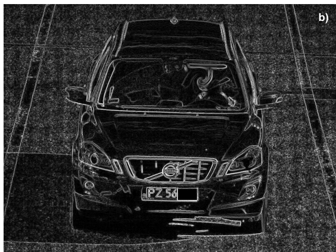
Fig. 1. A monochrome image (a) and the application of a filter detecting the edges (b) [2]
