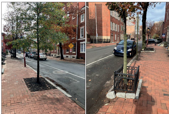
Fig. 5. Example of locating trees in a road lane in Philadelphia (USA)
