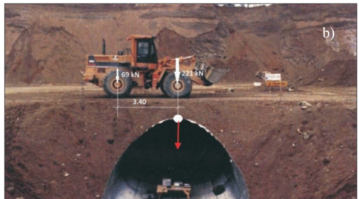
Fig. 1. Changes in deflection of the shell crown (a) of soil-shell structure (b) during a passage of a loader [5]
